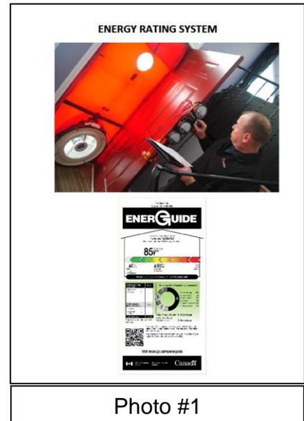
System. One way to determine this is to have a blower door test done. Have any of you had a blower door tests done in your own home? **(Show Photo #1 of the Energy Rating System)** A blower door test helps to show where heat is escaping your home and where cold air is getting in. It shows you where you can make changes to improve the energy efficiency of your home.
