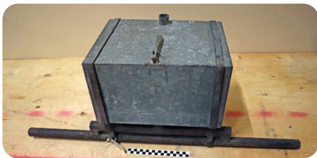
T.N.B. ice sprinkler for pebbling curling ice, WDM-1979-S-181
