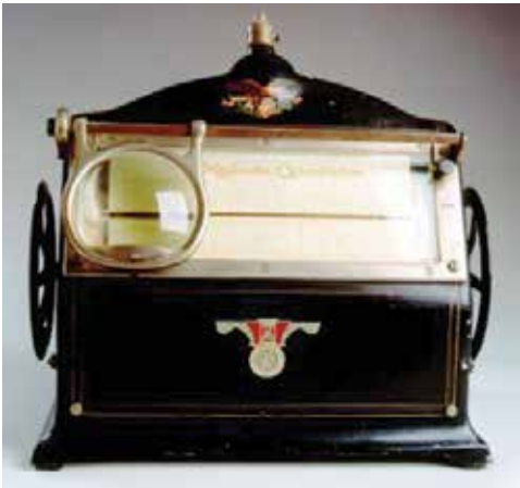
THE MEILICKE CALCULATOR FROM AROUND 1910 WAS USED TO CALCULATE INTEREST. IT PERFORMED NO CALCULATIONS ON ITS OWN BUT RATHER USED A SERIES OF TABLES TO TRACK INTEREST AND TAX RATES WDM-1979-S-123 C
