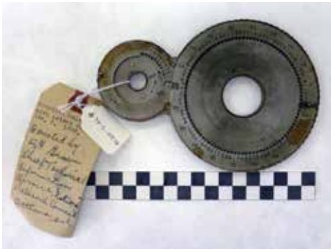
THIS 1895 DESK CALCULATOR USED TWO ROTATING DISCS TO PERFORM BASIC ARITHMETIC WDM-1973-S-10578
